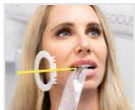
The ring shows the position of the sensor. It also has a guidance markings for centering the x-ray tube.
