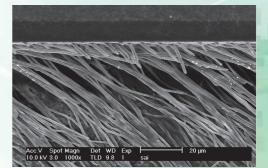
SEM image - Magx1000 \*\* In-house data, R&D, Tokuyama Dental Corporation. Note: This is a test model demonstrating hypersensitive dentin, using an extracted human tooth ground on the surface to expose the dentinal tubules.
